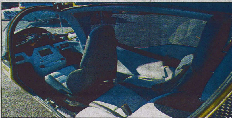
CAR-LIKE INTERIOR: The fully enclosed vehicle has two bucket seats, a floor-mounted brake, windows and even a windshield wiper.
